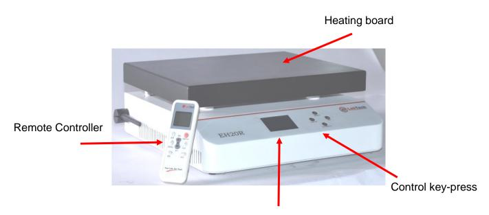
LCD display & Temperature Controller
