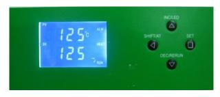
**SET** Set or check temperature, holding time and other parameters.
