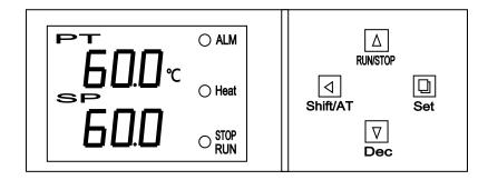
**SET** Set or check program step, temperature, holding time and other parameters.
